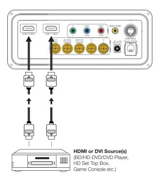
Figure 3-10. HDMI/DVI Source Connections
